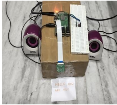
fig 5:- Circuit of speech assistive device for visually impaired people which consists of raspberry pi, pi camera, speakers
